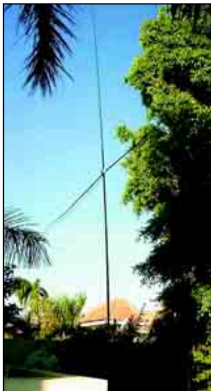
Figure 1—ST0P antennas in Khartoum. The DK9SQ loop is supported on a fiberglass pole—you can read more about this antenna at www.qsl.net/dk9sq/fibregle.htm .
